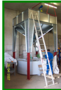
Buffer silo Rapeseed distributor Unfiltered oil tank with agitator
