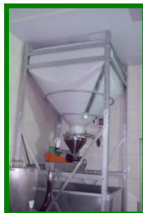
500 l buffer silo 4x60 l sedimentation vessels (stainless steel)
