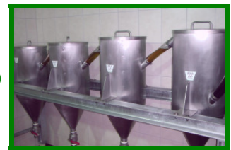
500 l buffer silo 4x60 l sedimentation vessels (stainless steel)
