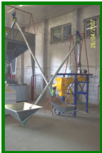
Rapeseed intake Cleaning system Magnetic separator 2 screw conveyors
